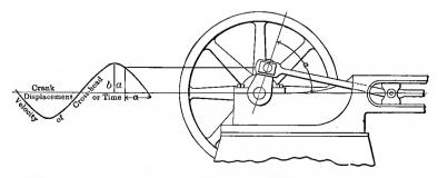
FIG. 40. Diagram showing relation of cross-head velocity of steam engine to annular velocity of crank.
